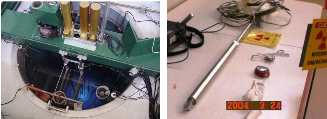
Figure 1. The IPR-R1 TRIGA Reactor and the instrumented fuel element
