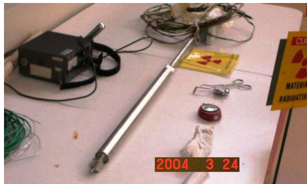
Figure 1. Instrumented fuel-moderator element
