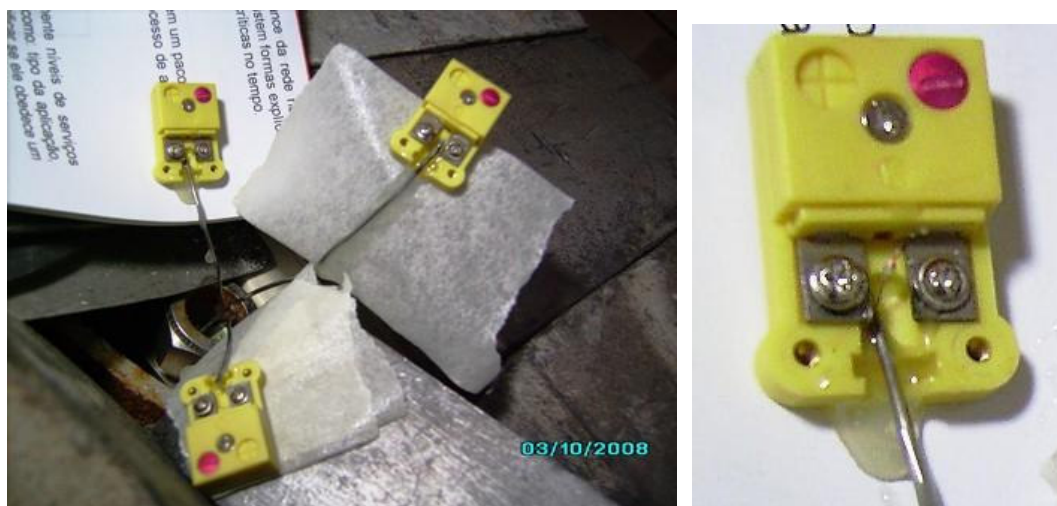
Fig. 9. Thermocouples wires fixed on the connectors
