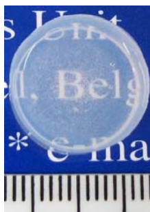
Figure 2. Fluorocarbon/silica composite, type I after drying at 150 °C.
