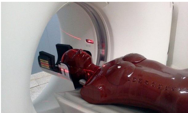
Fig. 1. Alderson Rando ® female anthropomorphic phantom positioned in the CT unit for absorbed dose measurements.
