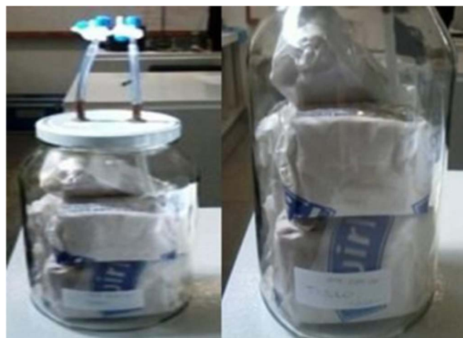
Fig. 1. Brick sample stored in a glass vessel to measure the 222 Rn concentration.
