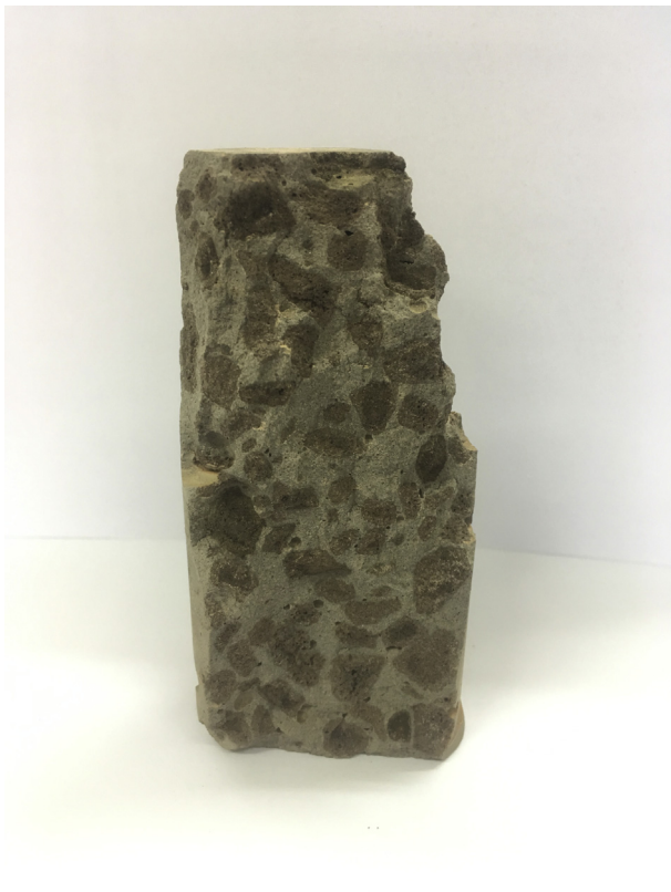
Fig. 9. Fracture surface of a concrete sample.
