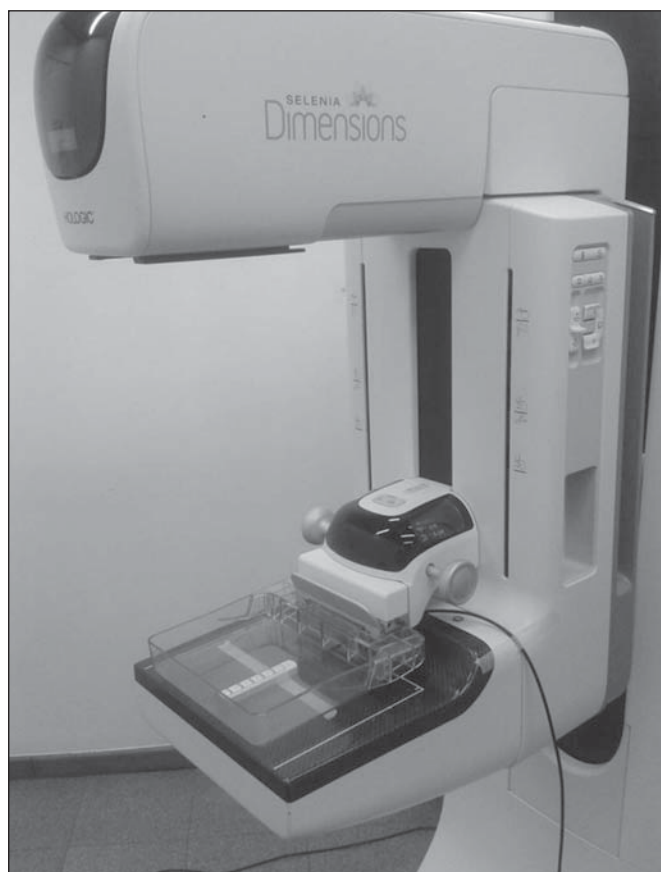
Figure 3. Experimental setup showing the compression plate in contact with detector.
