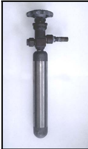
Fig. 2 Cylinder for radioactive gaseous tracer transport
