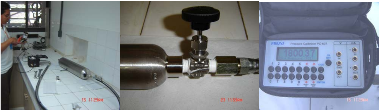
Figure 03 – Pressure test: cylinders, valves and hoses.
