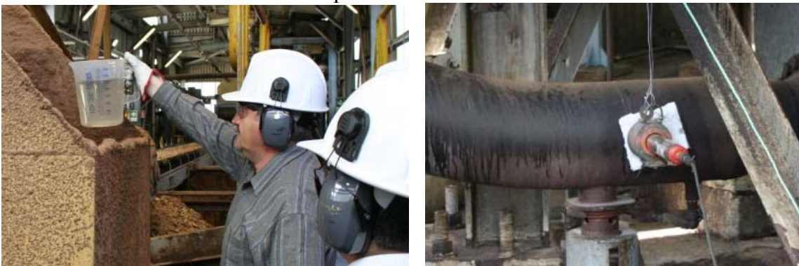
Figure 2: (a) Manual tracer injection at chip fill bin (b) Sensor placement in bottom blow line
