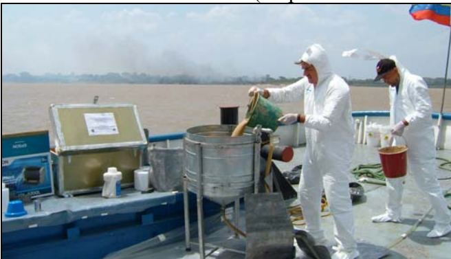
Figure 2 - Labelled mud mixer & injector Obs: the mud in the bucket is not yet labelled
