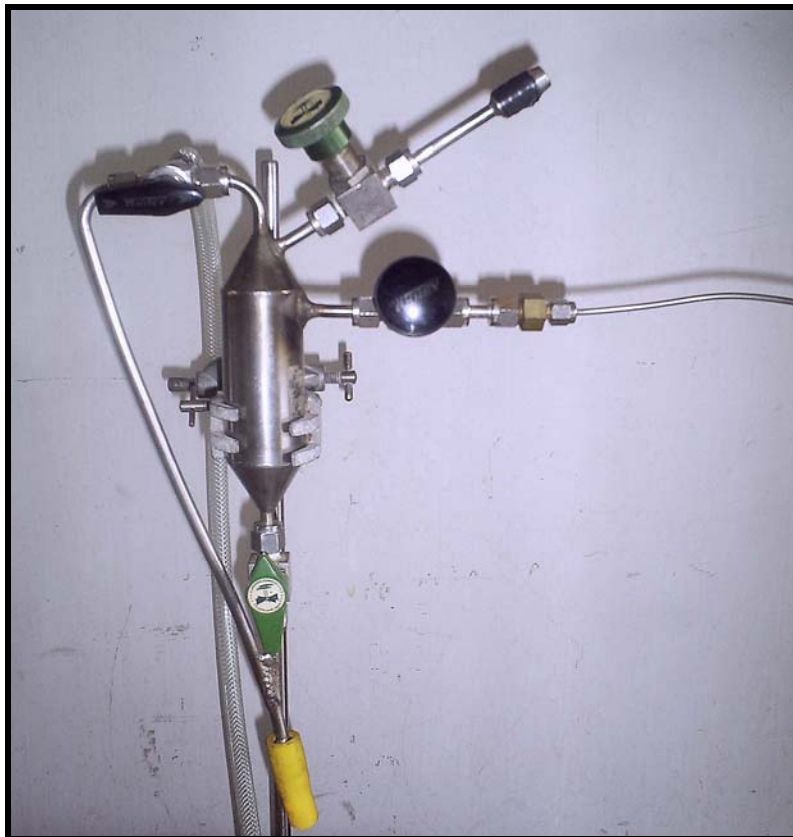
Fig. 4 Gas injection system
