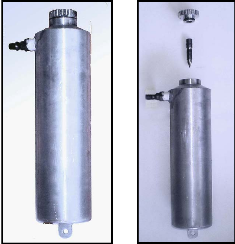
Fig. 1 Tank for gas storage and irradiation
