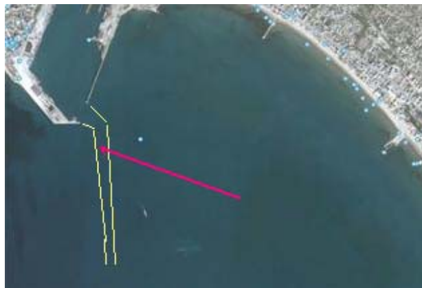
Fig. 5. Gulf of Durres, the harbour, the navigation channel and the main direction of sediment transport under the action of waves coming from the south-east.
