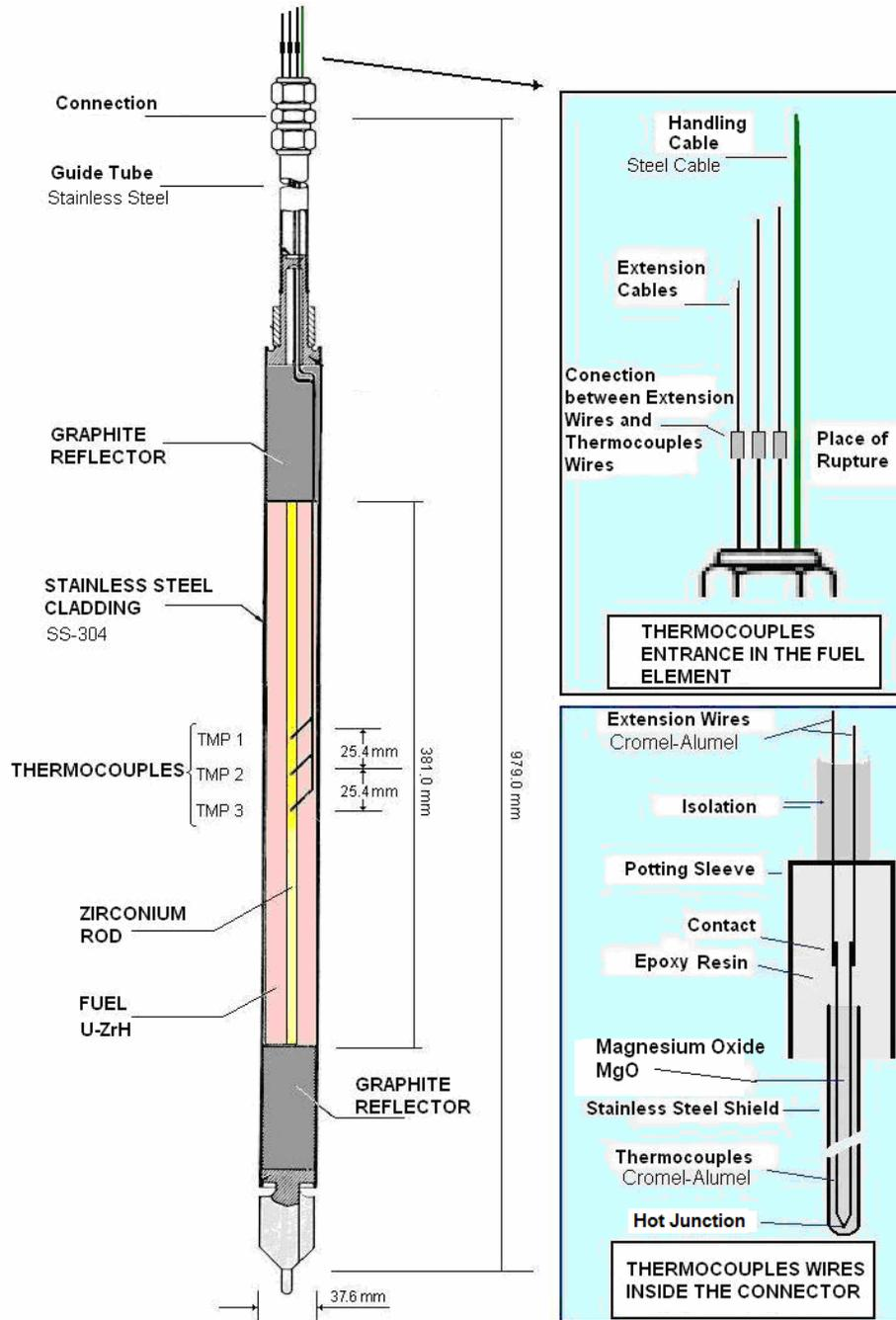
Figure 4. Instrumented fuel element and thermocouple connector detail
