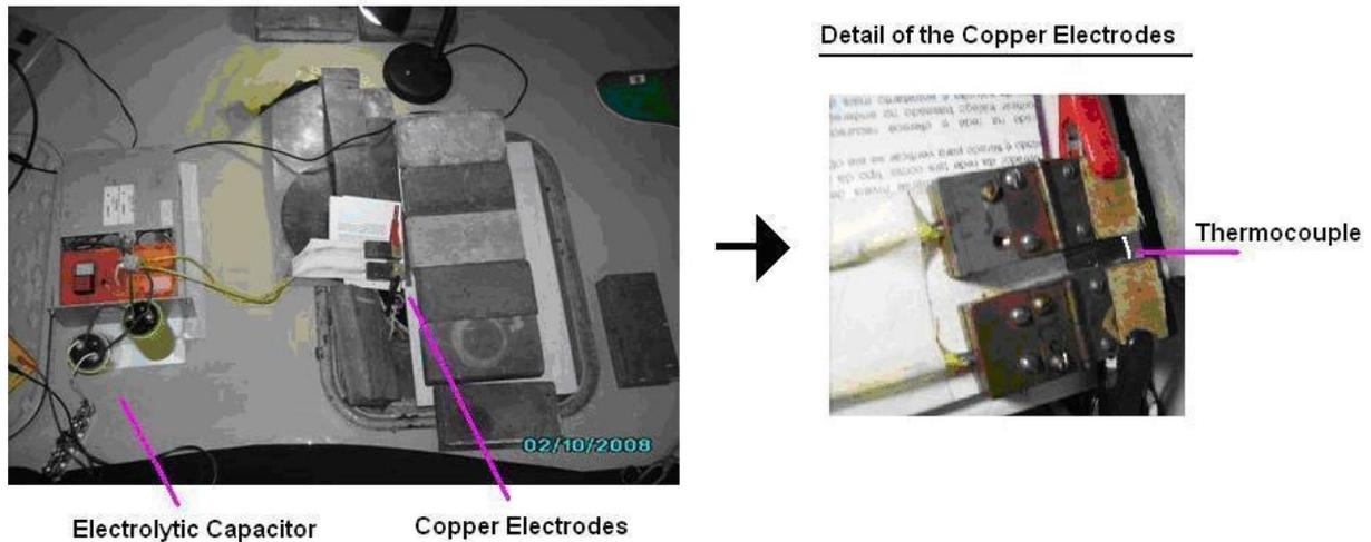
Figure 7. Assembly used for removal of the thermocouples shield by electric charge
