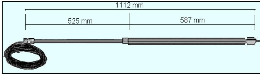
Figure 3. Instrumented fuel element (serial number 6821TC)
