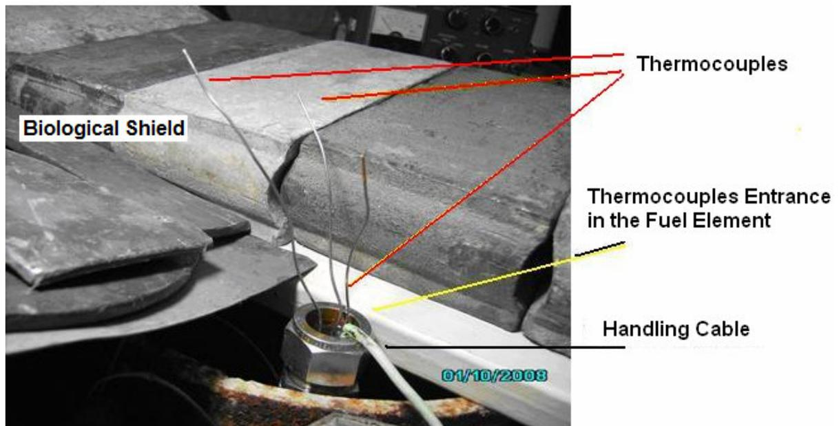
Figure 6. Place of the rupture of the thermocouples in the instrumented fuel element
