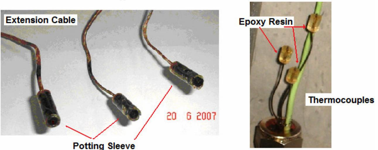
Figure 2. The thermocouples and extension cables after the breakdown
