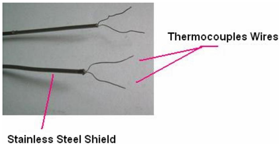
Figure 8. Two thermocouples after the shield and the MgO isolation had been removed
