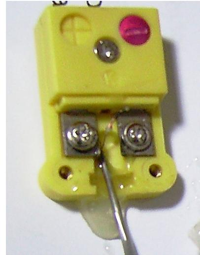
Figure 9. Thermocouples wires fixed on the connectors
