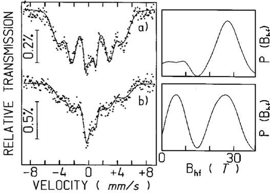
Fig. 3. Mössbauer spectra and the magnetic hyperfine field distributions,  $P(B_{\text{hf}})$ , of granular a)  $\text{Cu}_{91}\text{Fe}_9$  and b)  $\text{Cu}_{88}\text{Fe}_{12}$  samples measured at 5 K
