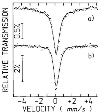
Fig. 7. Mössbauer spectra of a)  $\text{Cu}_{91}\text{Fe}_9$  and b)  $\text{Cu}_{88}\text{Fe}_{12}$  samples measured at 66 K
