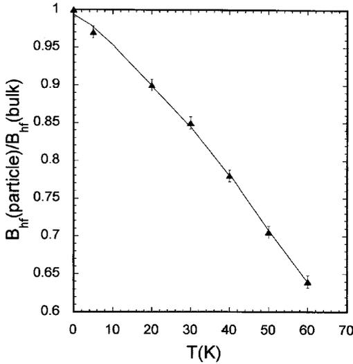
Fig. 6. Ratio of the magnetic hyperfine field of particles,  $B_{\text{hf}}(\text{particle})$ , to the magnetic hyperfine field of bulk,  $B_{\text{hf}}(\text{bulk})$ , vs. temperature
