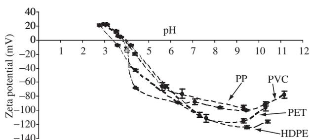
Figure 2. Zeta potential of planar surfaces of plastic materials.
