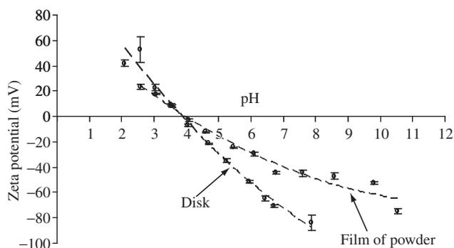
Figure 3. Zeta potential of a disk and a film of particles of black tourmaline.
