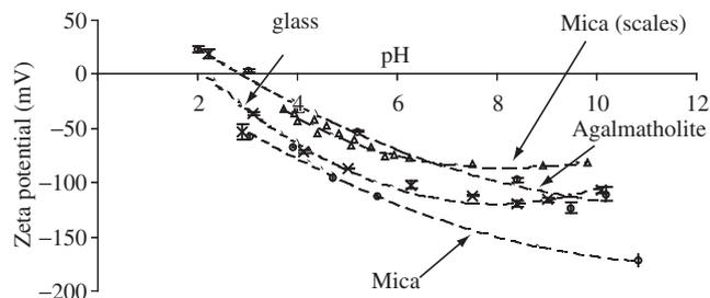
**Figure 4.** Zeta potential of disks of mica, glass and agalmatholite.
